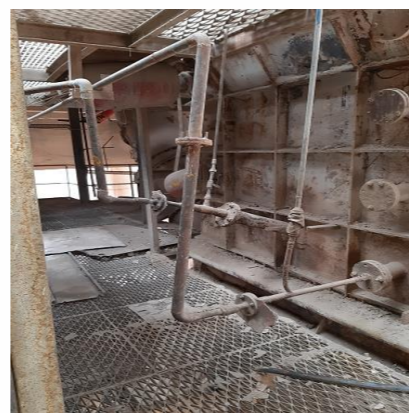
High NCV feeding point at reducing zone of calciner
